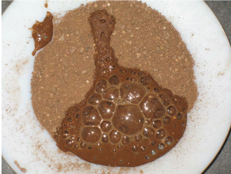
Figure 3. Test for the presence of soil carbonates by adding a drop of acid. Calcareous soils will produce carbon dioxide bubbles.
