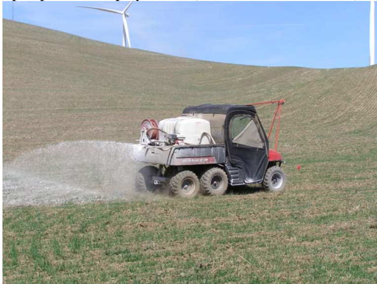
Figure 4. Lime application vehicle (ultra terrain vehicle) configured with a small holding tank, portable centrifugal pump, and one spray nozzle (Boom Buster nozzle 375).
