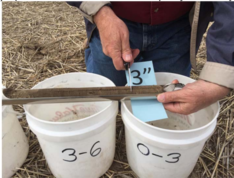
Figure 2. Soil sample probe soil cores are divided into sample layers for analysis.
