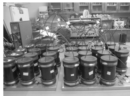
Figure 1: Semi enclosed system allowing capture of N gas emissions for sampling
