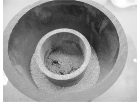
Figure 2: 4 cm (1.57 in) diameter PVC cylinder nested within the 7.75cm (3.1 in) cylinder with sand filling the medium to allow for air flow during sampling.
