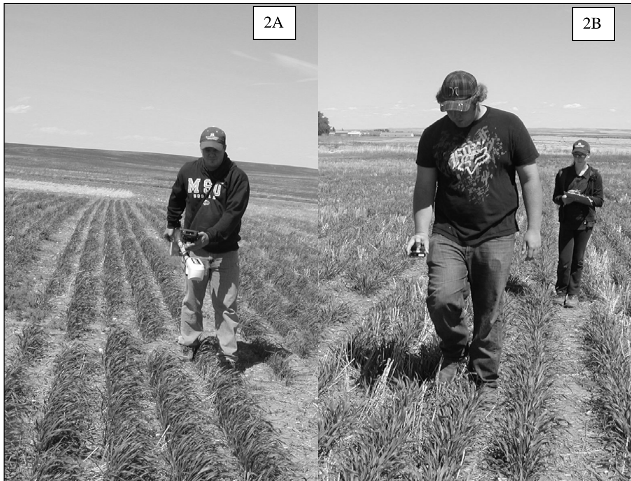
Figure 2. Robin Christiaens, Research Associate, and Jeff Jerome, Research Assistant, obtaining spring wheat reflectance measurements using GreenSeeker Sensor (2A) and Pocket Sensor (2B), Western Triangle Agricultural Research Center, Conrad, MT, Spring 2012.
