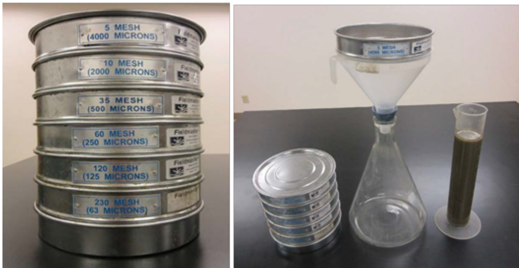
Figure 2. Stacked sieve set (left) and liquid dairy manure sieve filtration apparatus (right).
