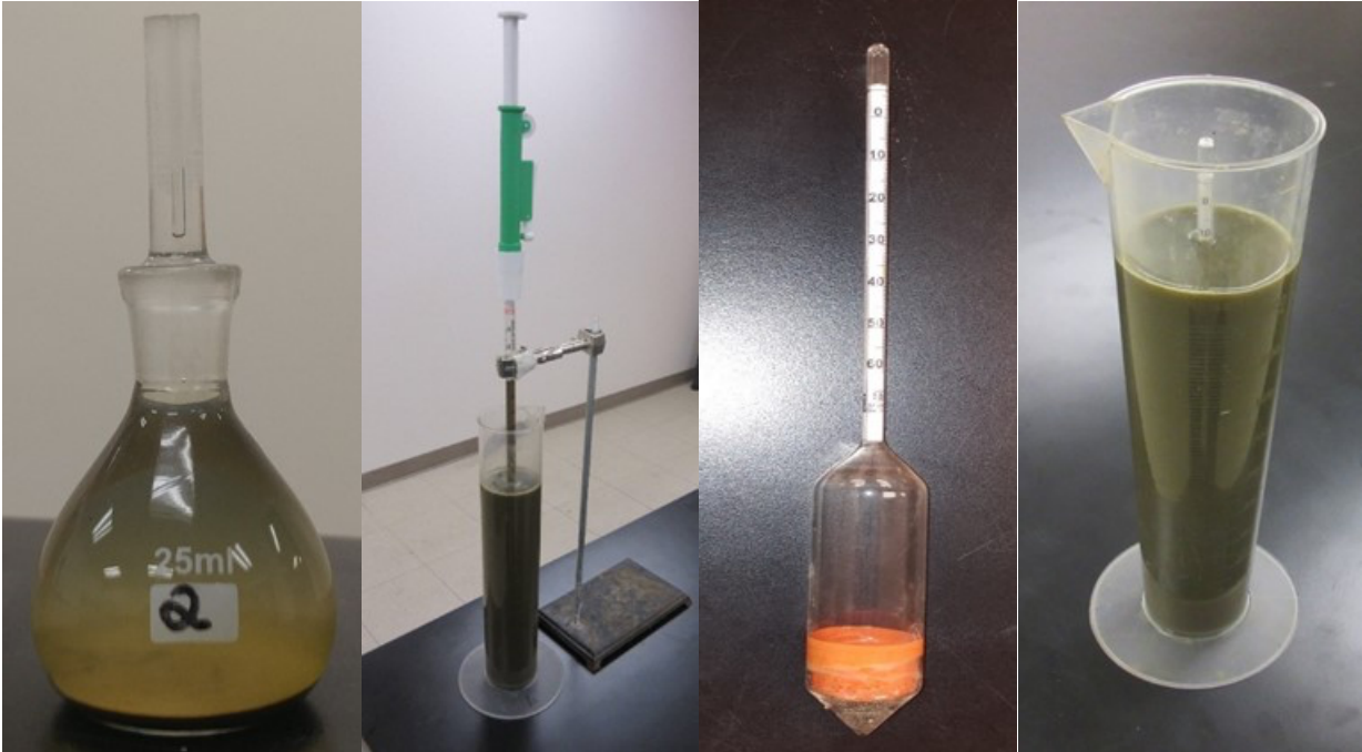
Figure 3. From left: pycnometer for particle density analysis, pipette method for extracting manure samples, ASTM 152-H hydrometer, hydrometer reading of the meniscus.
